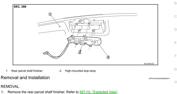
2. Remove the screws. And then remove the high-mounted stop lamp from the rear parcel shelf finisher.
