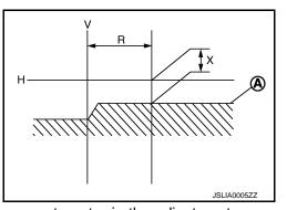
Adjust the cutoff line height (X) with the aiming adjustment screw so as to enter in the adjustment range 5. (M–N) according to the horizontal center line of headlamp (H).
