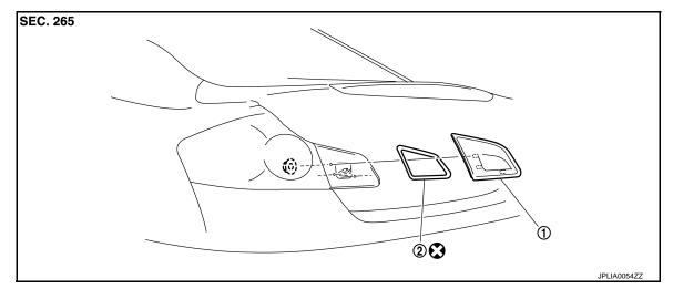
1. Back-up lamp2. Seal packingRefer to GI-4, "Components" for symbols in the figure.
